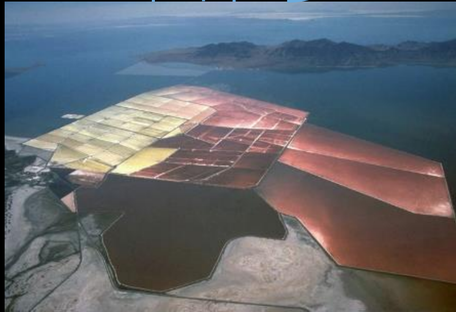
Salt water (brine) is concentrated in evaporation ponds
