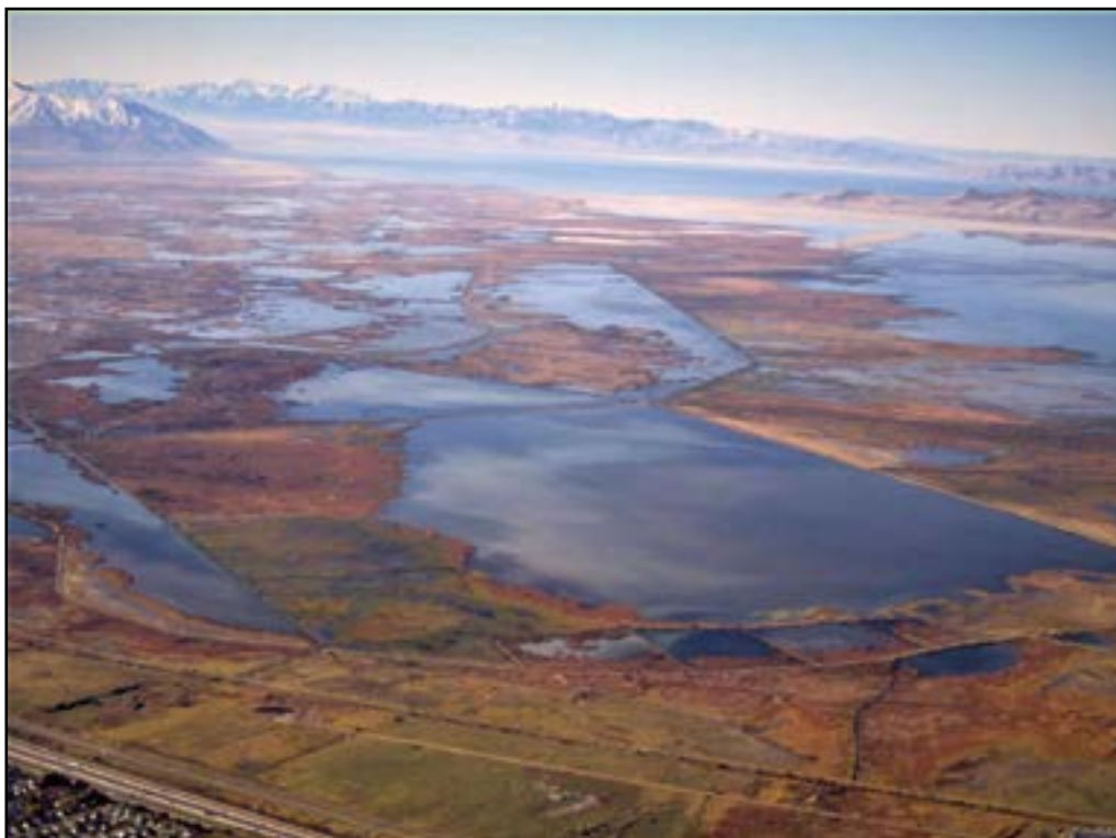
Aerial photograph of Farmington Bay WMA showing the extensive dike system used to control water. Typical of many wetlands around the GSL. Courtesy Utah Division of Wildlife Resources.
